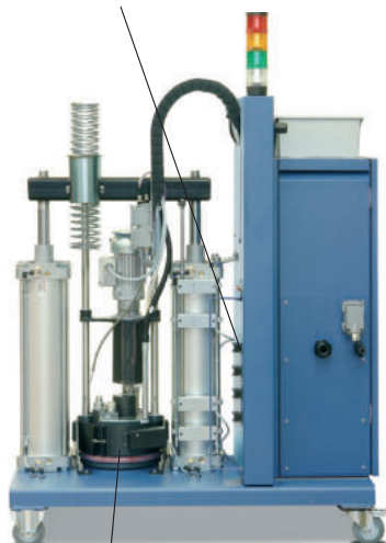
Four additional temperature channels for control of spray guns, heaters, etc.
