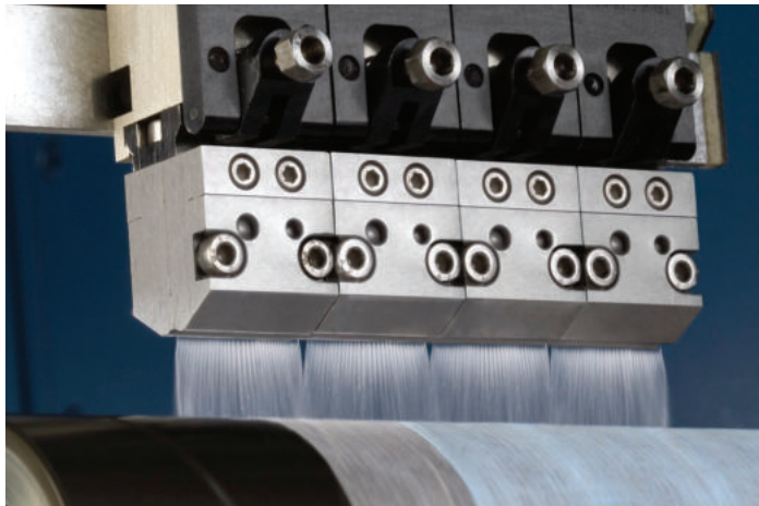
Universal Control Coat nozzles produce consistent patterns in machine and cross-web directions.
