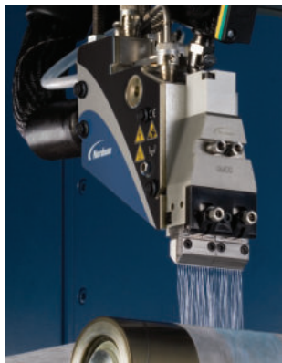
Wide Universal UM50 modules require fewer modules to cost-effectively meet the demands of continuous laminating applications.
