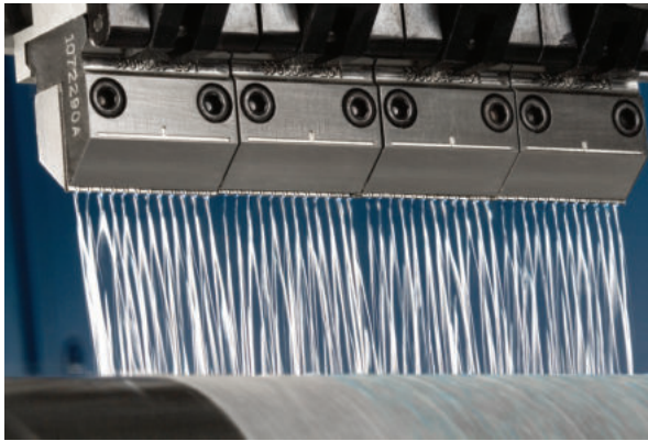
A greater nozzle-to-substrate distance decreases exposure to airborne contaminants that can compromise performance.
