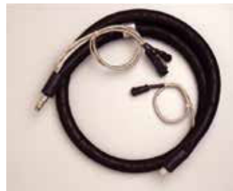
Handgun end of hose has one cordset. Melter end has standard cordset to melter, and second cordset for optional air control kit for swirl and spray patterns.
