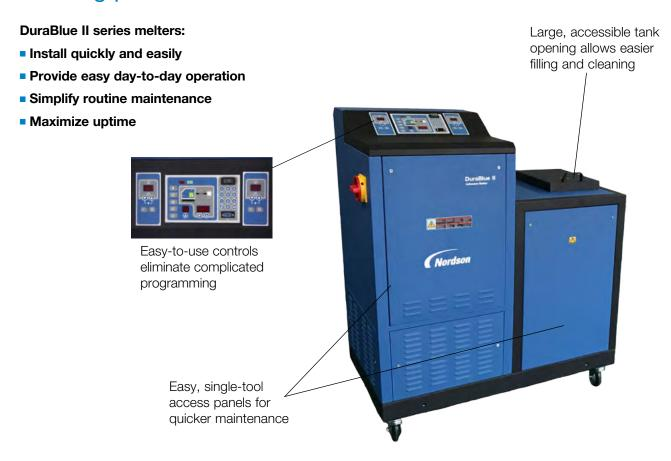
Nordson DuraBlue II series melters are designed to deliver hot melt adhesive in support of low to mid-speed production. The metering spur-gear pumps with variable-speed AC motors and key-to-line functionality satisfies a wide range of manufacturing requirements. A non-stick coated tank and reservoir design reduces adhesive degradation while maximizing adhesive throughput. The versatile control panel offers a choice of programming methods using either the keypad or arrow keys.
